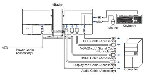
\* VGA (D-Sub) cable is not supplied with the monitor; you need to use a special VGA (D-Sub) cable dedicated for this model. Please contact the iiyama Support Centre in your country if you wish to connect the monitor via the VGA input.
