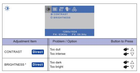
\* Adjust the Brightness when you are using the monitor in a dark room and feel the screen is too bright.
