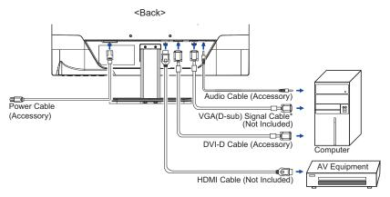
\* VGA (D-Sub) cable is not supplied with the monitor. If you use low quality VGA (D-Sub) cable, it may cause a result of electro-magnetic interference. Please contact the iiyama Support Centre in your country if you wish to connect the monitor via the VGA input.
