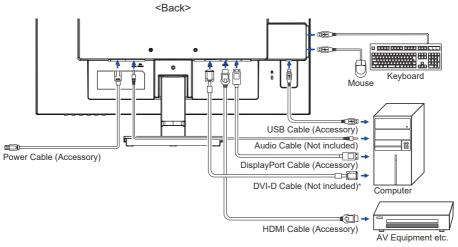
\* DVI dual-link cable is not supplied with the monitor. If you use low quality DVI dual-link cable, it may cause a result of electro-magnetic interference. Please contact the iiyama Support Centre in your country if you wish to connect the monitor via the DVI input.
