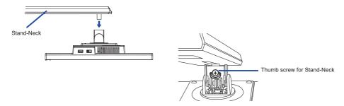
3 Use the 'thumb screw' provided to secure the base to the monitor.
