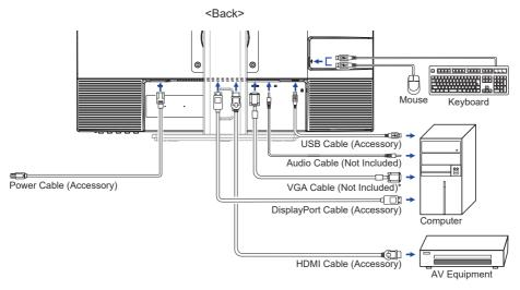
\* VGA cable is not supplied with the monitor. If you use low quality VGA cable, it may cause a result of electro-magnetic interference. Please contact the iiyama Support Centre in your country if you wish to connect the monitor via the VGA input.
