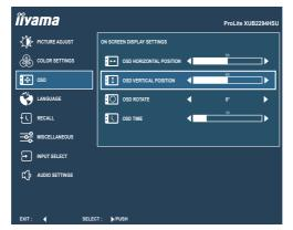
Press or tilt the Joystick  $[\langle 2 \rangle - \langle 2 \rangle]$  and finally tilt it  $[\langle 2 \rangle]$  to close the On Screen Display feature. All changes are saved in the memory.
