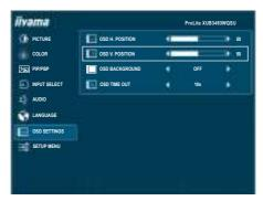
When you press the EXIT Button to end the adjustment, all changes are saved in the memory.
