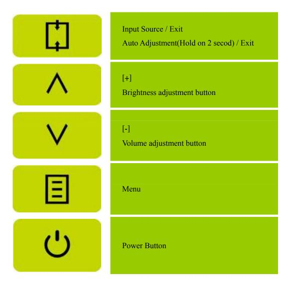
Figure.4. Control Panel Buttons
