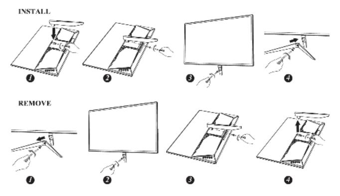
Figure.1. Installing and Removing the Base
