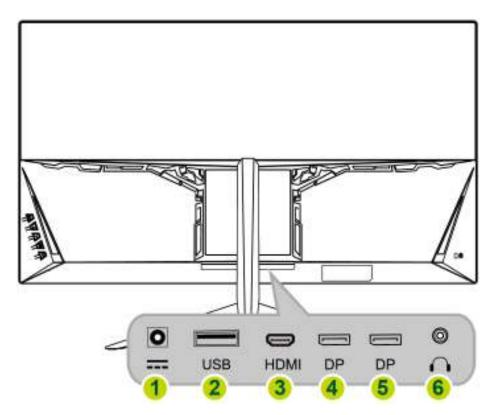
Figure.2. Connecting to a PC
