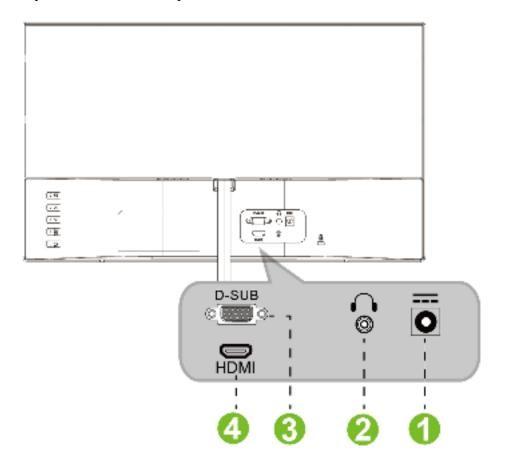
Figure.2. Connecting to a PC
