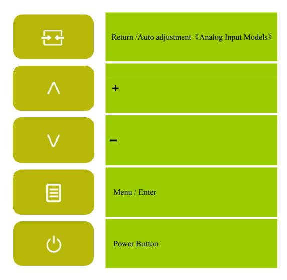
Figure.4. Control Panel Buttons
