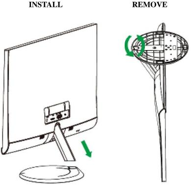
Figure.1. Installing and Removing the Base
