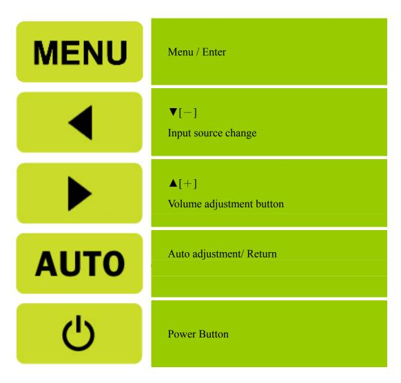
Figure.4. Control Panel Buttons
