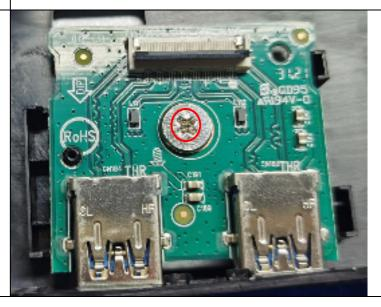
Remove the screw on the usb board
