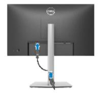
**3.** Connect the DisplayPort, USB Type-C, or HDMl cable from your monitor to the computer.
