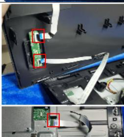
open the cover on the keyboard/ usb board and then pull out the cables
