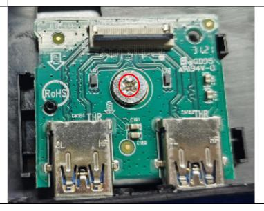
Remove the screw on the usb board
