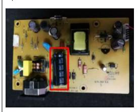
Take out the capacitor pin solder with soldering iron.
