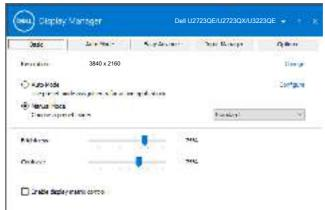
NOTE: When multiple Dell monitors are connected, select "Enable display matrix control" to apply brightness, contrast and color presets controls to all monitors.
