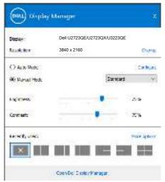
The **Quick Settings** dialog box also provides access to Dell Display Manager's advanced user interface that is used to adjust basic functions, configure auto mode and access other features.
