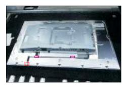
Use a Philips-head screwdriver to remove 4pcs screws for unlocking the bracket with the panel.
