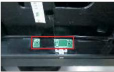
S13 Disconnect the panel lamp cables away from the two connector of the panel, and then release the lamp cable by tearing off the tapes.
