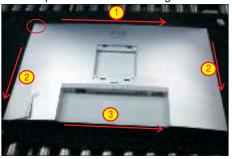
S7 Lift the rear cover up carefully. Disconnect the joystick key cable from the connector of the interface board, and then remove the rear cover and put it aside for later disassembling.
