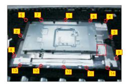
Disconnect the LED cable from the connector of the interface board, and then tear off the tapes on the back of the back.
