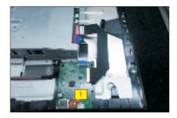
Use a Philips-head screwdriver to remove 14(9+5)pcs screws for locking the middle bezel with the panel, then tear off 1pcs aluminum foil for releasing the LED cable.
