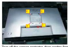
Tear off the screen protector, then wedge fingers between rear cover and the middle bezel on the corners of the top side of the monitor to release the rear cover, then use one hand to press the middle bezel, the other hand to pull up the rear cover in order of arrow preference for unlocking the rear cover.
