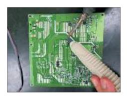
S20-5 Lift the bulk cap. up and away from the PCB.
