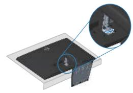
**3.** Slide the stand out of the monitor completely.
