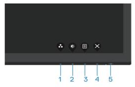
1. Press and hold Button 4 for four seconds, a menu appears on the screen.
