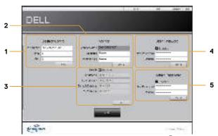
Configures the settings between the monitor and Crestron® control system. Click the **[Exit]** button to return to the Main window.
