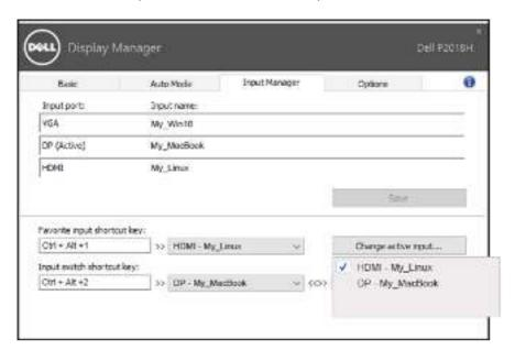
NOTE: DDM communicates with your monitor even when the monitor is displaying video from another computer. You can install DDM on the PC you frequently use and control input switching from it. You may also install DDM on other PCs connected to the monitor.
