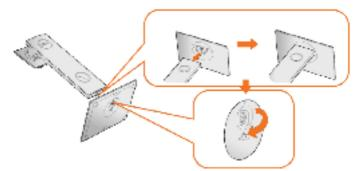
5 Lift the cover, as shown, to expose the VESA area for stand assembly.
