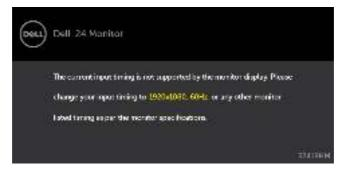
This means that the monitor cannot synchronize with the signal that it is receiving from the computer. See Monitor Specifications for the Horizontal and Vertical frequency ranges addressable by this monitor. Recommended mode is  $1920 \times 1080$ .
