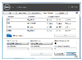
You can assign a USB upstream port with your video input. The assigned USB upstream
