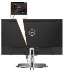
7 Insert the cable holder attached on the speaker cable into the stand slot. Adjust the cable holder position along the slot accordingly.
