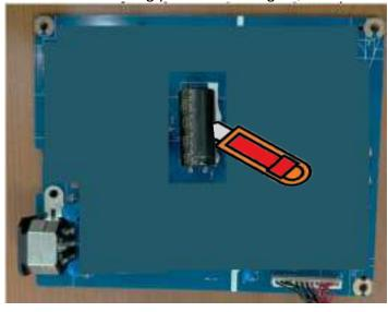
S20-3 Take out bulk cap. pin solder with soldering iron and absorber
