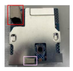
S11 Disassemble "USB board" from "USB Shielding"
