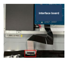
Attach a yellow tape to fix "LVDS FFC" on "Panel"
