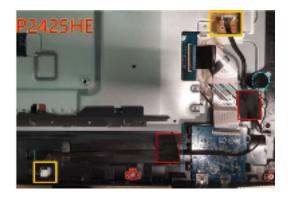
S16 Insert "Control board FFC" to "Control board"
