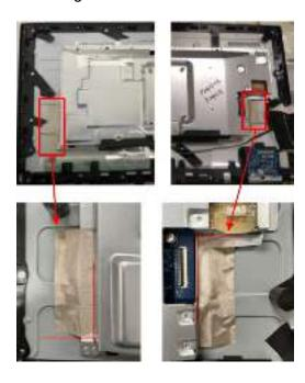
S13 Tear off an aluminum foil and a yellow tape from "LVDS FFC" on "Panel"
