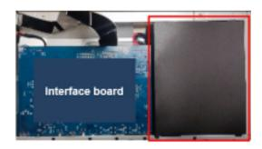
Attach two acetate tapes to cover the convex holes on "Panel"
