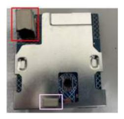
S14 Assemble "USB board" with "Middle Frame"
