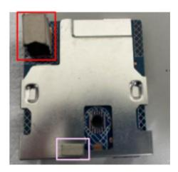
S11 Disassemble "USB board" from "USB Shielding"
