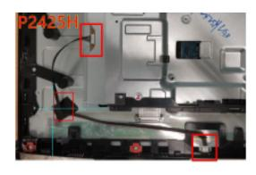
Assemble "USB board" with "USB Shielding"
