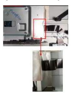
S14 Insert "Control board FFC" to "Control board"
