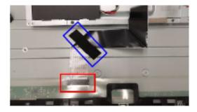
Sa Attach 3 conductive tapes on "Main Shielding and "Panel"
