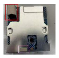
S11 Disassemble "USB board" from "USB Shielding"
