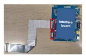
Assemble "Interface board" to "Main Shielding"
