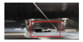
Unlock 3 screws to disassemble "Control board" from "Rear Cover"
