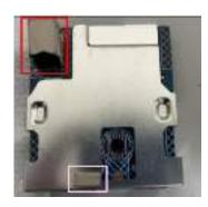
S11 Disassemble "USB board" from "USB Shielding"
