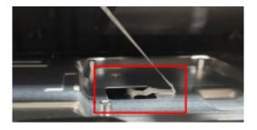
Unlock 3 screws to disassemble "Control board" from "Rear Cover"
