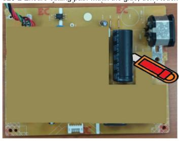
S20-3 Take out bulk cap. pin solder with soldering iron and absorber
