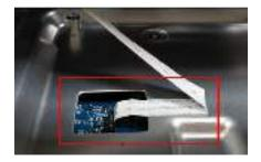
Unlock 3 screws to disassemble "Control board" from "Rear Cover"
