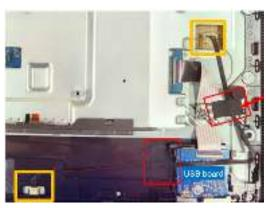
Tear off a black tape from "USB board FFC" and "Panel
