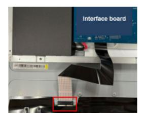
S8 Attach a yellow tape to fix "LVDS FFC" on "Panel"
