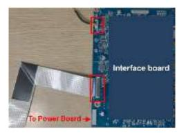
**S18** Remove electrolyte capacitors (red mark) from printed circuit boards
