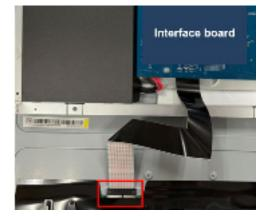
**S14** Unlock 13 screws to disassemble "Middle Frame" from "Panel"
