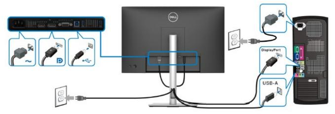
Connect/ disconnecting the HDMI cable (optional), USB 3.2 upstream cable and Power cable
