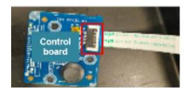
S13 Assemble "Control board" to "Rear Cover"
