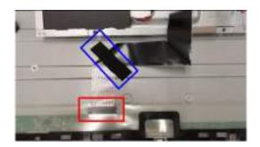
S13 Unlock 13 screws to disassemble "Middle Frame" from "Panel"
