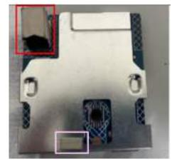
**S10** Disassemble "USB board" from "USB Shielding"
