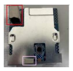
S11 Disassemble "USB board" from "USB Shielding"
