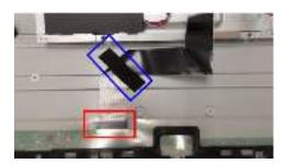
Attach 3 conductive tapes on "Main Shielding and "Panel"
