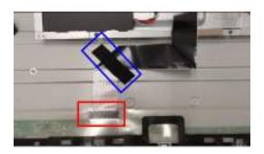
Unlock 13 screws to disassemble "Middle Frame" from "Panel"
