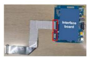
Assemble "Interface board" to "Main Shielding"
