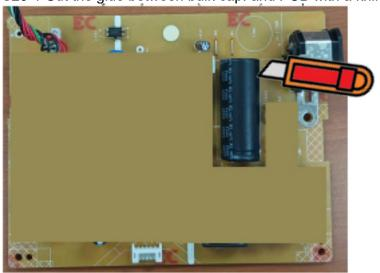
S20-2 Ensure cutting path within the glue, don't touch bulk cap. or PCB
