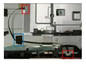
S10 Assemble "USB board" with "USB Shielding"
