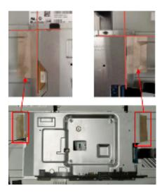
Insert "Backlight wire" to "Panel" and "Power Board"
