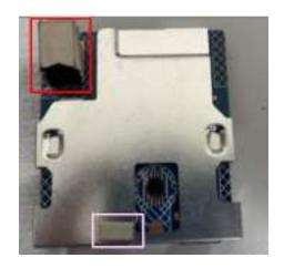
S10 Disassemble "USB board" from "USB Shielding"
