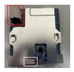
S10 Disassemble "USB board" from "USB Shielding"
