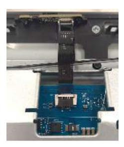
S11 Unplug "Ambient Light Sensor FFC" from "Sensor board"
