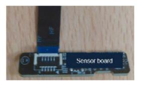
S14 Assemble "Sensor board" into "Middle Frame"
