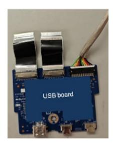
Assemble "USB board" to "Middle Frame" and fix it by screw\*1
