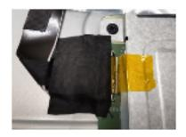
Place "Main Shielding" on "Panel" and S9 lock 4 screws to fix it on "Panel"
