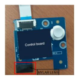
Assemble "Control board" to "Rear Cover" and fix it by screws\*3
