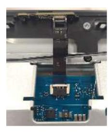
Assemble below mylars to "Main Shielding"
