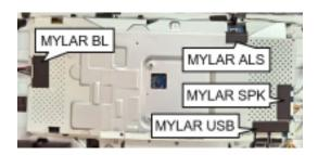
S10 Unplug "Ambient Light Sensor FFC" from "Interface board"
