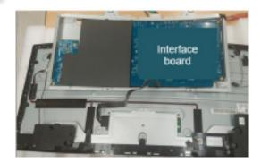
S19 Unlock 19 screws to disassemble "Middle Frame" from "Panel"
