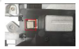
S15 Unlock 4 screws to disassemble "Main Shielding" from "Panel"
