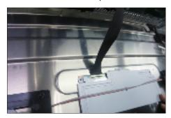
Lift up the middle frame and put it into a fixture, tear S15 off all the cable tape and the mylar tape for releasing the LED key board away from the middle frame.
