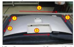
Lift up the rear cover, and disconnect the joystick cable and sensor cable away from the connectors, and then remove the rear cover and put it aside.
