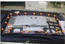
Tear off 3pcs aluminum foil, then use a Philips-head screwdriver to remove 4pcs screws for locking the bracket chassis module with the panel.
