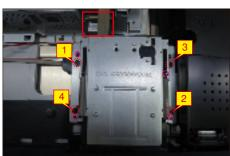
Use a Philips-head screwdriver to remove 1pcs screw for releasing the USB unit, then remove the USB cover, then use a Philips-head screwdriver to remove 1pcs screw for locking the USB board. Disconnect the USB connective cable.
