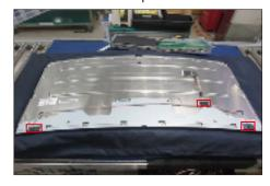
Remove the mylar sheet from the hooks of the main **S17** bracket chassis.
