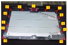
Lift up the middle bezel away from the pane module, S17 then put it on a cushion foam for later disassembling.
