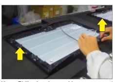
Use a Philips-head screwdriver to remove 4pcs screws for unlocking the left and right Mic boards S18 with the middle frame, then release the two Mic boards away from the middle frame.
