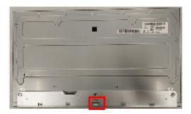
S18 Disassemble 2 plastic BOSS from panel
