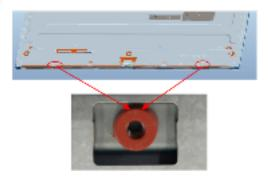
S19 Disassemble mylar from Main SHD
