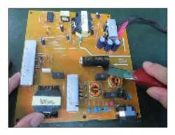
S23-4 Take out bulk cap. pin solder with soldering iron and absorber.
