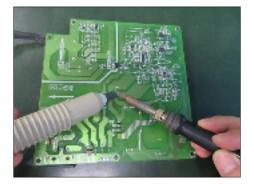
S23-5 Lift the bulk cap. up and away from the PCB.
