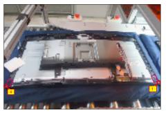
Use a Philips-head screwdriver to remove 1pcs screw for unlocking the USB board, then disconnect the USB cable and touch cable away from the connectors of main board. Release the USB board away from the hook of the middle frame. (No.1 screw size=M3x3.5, Torque=4±0.5 kgfxcm)
