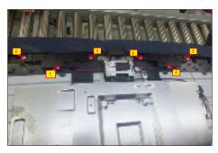
Tear off 1pcs tape, then disconnect the speaker cable away from the board, then release the speakers from the probers of the middle frame. Disconnect the panel lamp cable away from the connectors of the main board and panel, then release the panel lamp cables from the hooks of the middle frame.
