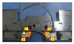
Release the touch key cable away from the panel, S19 then disassemble the front bezel with the panel, then tear off the mylar tape and release the touch board.
