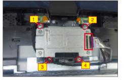
Use a Philips-head screwdriver to remove 4pcs screws for unlocking the bracket chassis with the
