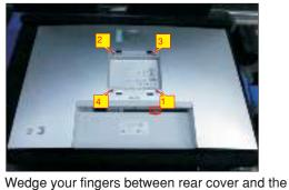
middle bezel on the corners of the top side of the monitor to release the rear cover, then use one hand to press the middle bezel, the other hand to pull up carefully the rear cover in order of arrow preference for unlocking mechanisms of rear cover.
