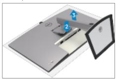
Put the monitor on a protective cushion, then use a Philips-head screwdriver to remove 4pcs screws for unlocking mechanisms. Remove DP caps.
