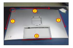
S6 Lift the rear cover up carefully. Disconnect the joystick key cable from the connector of the interface board, and then remove the rear cover and put it aside for later disassembling.
