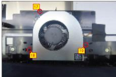
Use a Philips-head screwdriver to remove 16pcs screws for unlocking the middle frame with the panel, then tear off 3pcs tapes and disconnect fans' wire and touch wire from the connectors, and then remove the fan from the hook of the middle frame.
