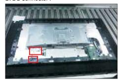
Use a Philips-head screwdriver to release one screw for unlocking the USB board, and disconnect the two cables, then release the USB board from the hooks of the middle bezel.
