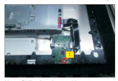
Use a Philips-head screwdriver to remove 18(13+5)pcs screws for unlocking the middle bezel with the panel module.
