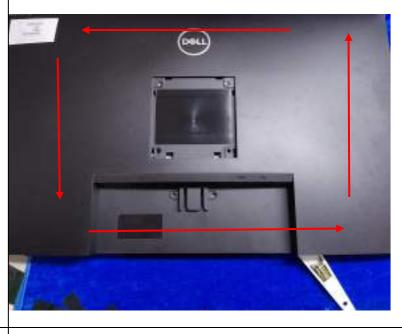
Use scraper to insert from the bottom site and then open the rear cover
