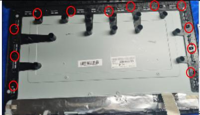
Remove the screws on the middle frame
