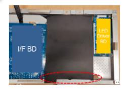
Unlock 10 PCBA screws to disassemble "I/F BD", "SPS BD" and "LED Driver BD" from Main SHD
