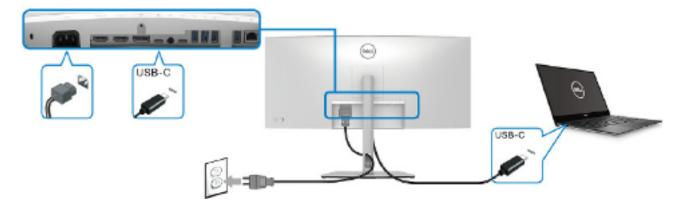
Connecting/ disconnecting the super speed USB 10 Gbps (USB 3.2 Gen2) cable and Power cable
