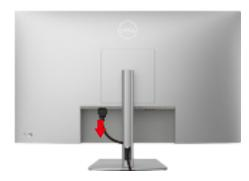
Remove stand from the product.(Press the stand release button, lift the stand up and away from the monitor)
