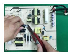
S20-2 Ensure cutting path within the glue, don't touch bulk cap. or PCB.
