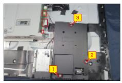
Use a Philips-head screwdriver to remove 4pcs screw for unlocking the USB unit with the middle frame, and then release the USB unit from the hooks of middle frame.
