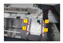
Use a Philips-head screwdriver to remove 2pcs screws for unlocking the USB cover, remove the USB cover, then use a Philips-head screwdriver to remove 1pcs screw for locking the USB board with the USB bracket. Disconnect the USB connective cable.
