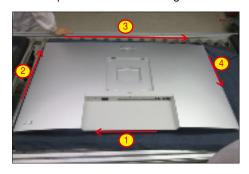
S6 Lift the rear cover up carefully. Disconnect the joystick key cable from the connector of the interface board, and then remove the rear cover and put it aside for later disassembling.
