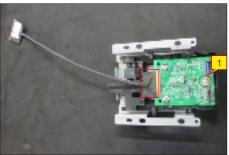
S11 Release the speakers' cable to from the hooks of the middle frame, then remove the speakers.
