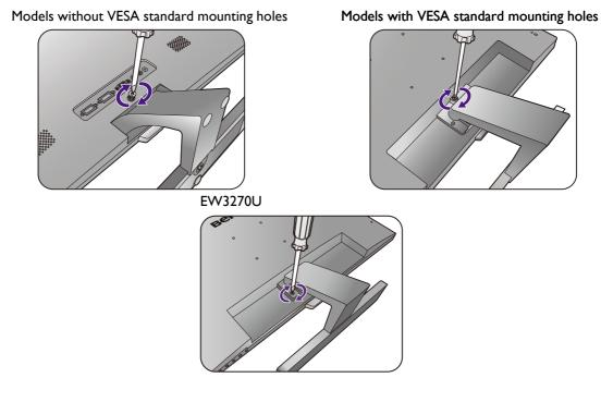
To secure or release a screw, a flat-head screwdriver or a coin is required.
