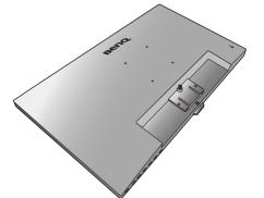
Attach the monitor stand to the monitor base as illustrated until it locks in place.
